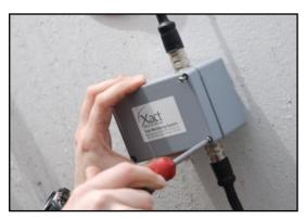
Use a #2 Philips screw driver to remove the Xact Communication Box cover. The four screws are captured in the lid to prevent accidental loss while opened. It may be convenient to only loosen and not fully unscrew one of the four screws, allowing the lid to be rotated out of the way.
