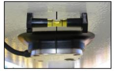
Push upward firmly in the center of the Sensor and hold for about 10 seconds to ensure that the acoustic gel is evenly distributed between the wall of the tank and the face of the Sensor.
