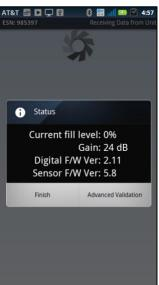
The Xact system will measure the tank fill level and display it here. Select **Finish** when complete. Once complete, exit the Xact application, remove the Bluetooth adapter, and replace the Xact Communication Box cover. Before you leave, ensure that the cover is tightly sealed.
