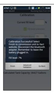
Progress of the Calibration is indicated by the bar, and should complete in about 2-6 minutes. The application indicates if the calibration cycle was successful or not by displaying the appropriate screen.
