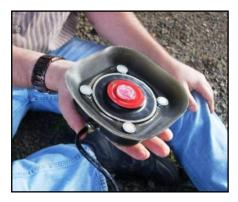
Apply the complete contents of the provided pre-measured packet of acoustic gel to the center of the lens face of the Sensor as shown in the picture. The amount of gel applied is critical to function, so use the entire gel package contents. If you ever need to remove and re-install the Sensor, ensure that both surfaces are wiped clean, then re-apply the pre-measured amount of acoustic gel from a new package.
